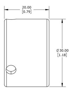
LIKA ELECTRONIC REDUCER BUSHING, 30mm TO 1IN, METAL, FOR USE WITH LIKA ELECTRONIC A80 SERIES ENCODERS, MOUNTING HARDWARE INCLUDED
