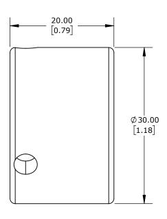
LIKA ELECTRONIC REDUCER BUSHING, 30mm TO 20mm, METAL, FOR USE WITH LIKA ELECTRONIC A80 SERIES **ENCODERS, MOUNTING HARDWARE INCLUDED**
