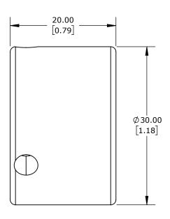
LIKA ELECTRONIC REDUCER BUSHING, 30mm TO 5/8IN, METAL, FOR USE WITH LIKA ELECTRONIC A80 SERIES ENCODERS, MOUNTING HARDWARE INCLUDED
