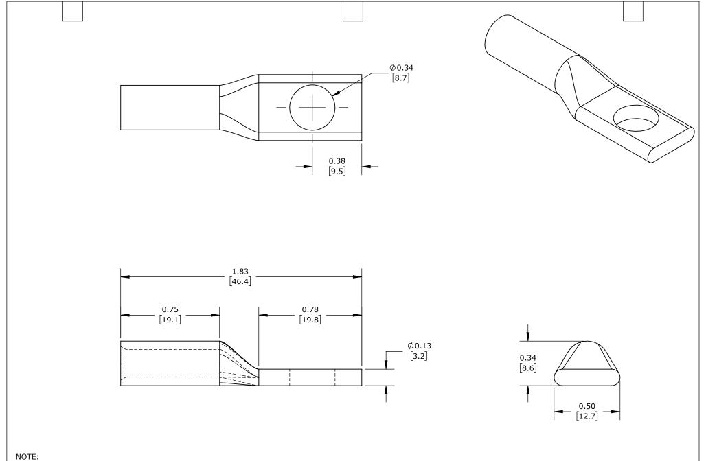
NOTE: FOR CORRECT CABLE SELECTION AND SIZING, PLEASE REFER TO THE PENN-UNION INSERT / STUFFER SHEET
