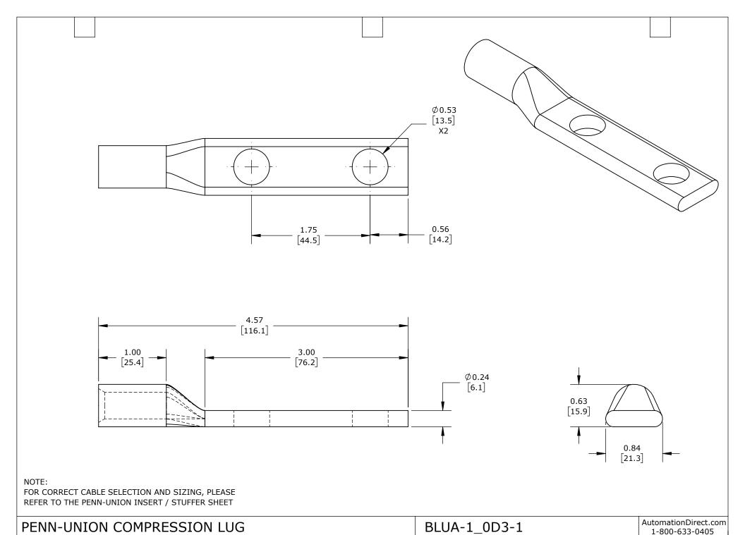
3rd NOT TO PART DIMENSIONS MAY DIFFER SLIGHTLY INCH UNITS USED FOR UNLESS OTHERWISE inch ANGLE SCALE DUE TO MANUFACTURER'S VARIANCES PART DESIGN SPECIFIED UNITS ARE: [mm] REV. -- 8/18/2025 SHEET 1 OF 1
