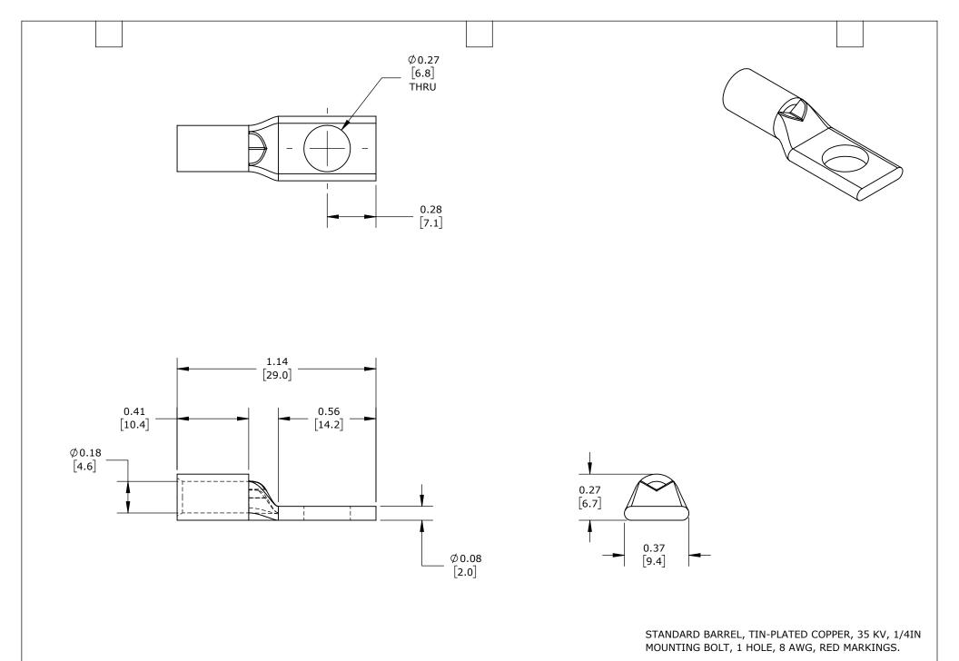
BLU-8S15-1 AutomationDirect.com PENN UNION COMPRESSION LUG 1-800-633-0405 PART DIMENSIONS MAY DIFFER SLIGHTLY UNLESS OTHERWISE inch LATEST VERSION NOT TO INCH UNITS USED FOR 3rd SHEET 1 OF 1 SPECIFIED UNITS ARE: ANGLE DUE TO MANUFACTURER'S VARIANCES [mm] 9/9/2024 SCALE PART DESIGN
