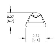
STANDARD BARREL, TIN-PLATED COPPER, 35 KV, #10 MOUNTING BOLT, 1 HOLE, 8 AWG, RED MARKINGS.
