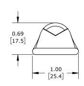
STANDARD BARREL, TIN-PLATED COPPER, 35 KV, 1/2IN MOUNTING BOLT, 1 HOLE, 4/0 AWG, PURPLE MARKINGS.
