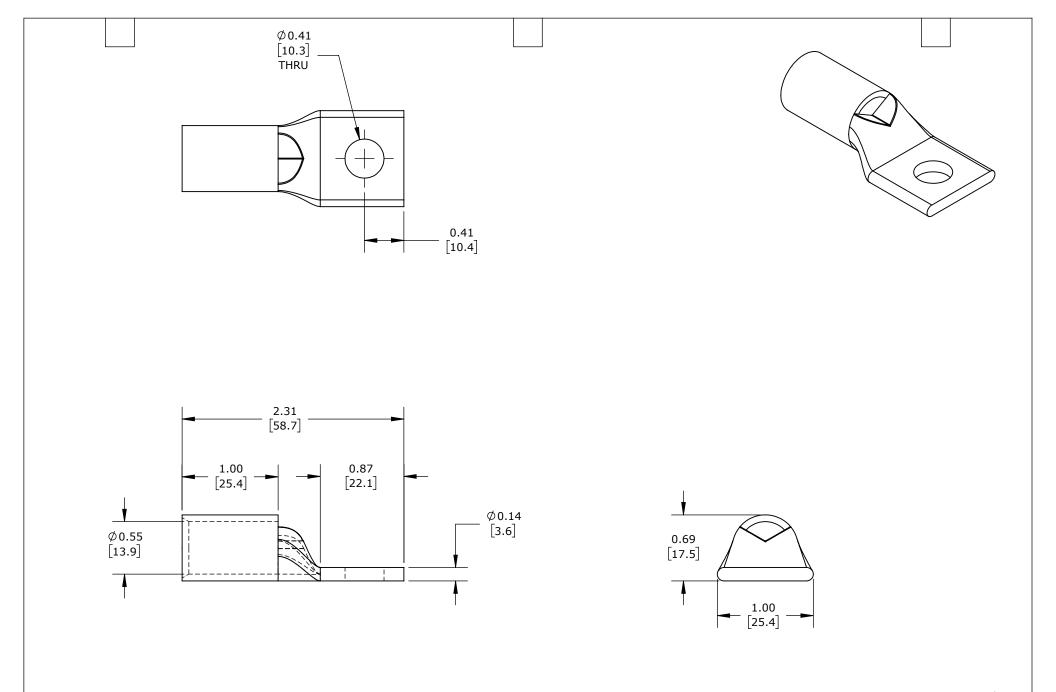
STANDARD BARREL, TIN-PLATED COPPER, 35 KV, 3/8IN MOUNTING BOLT, 1 HOLE, 4/0 AWG, PURPLE MARKINGS.
