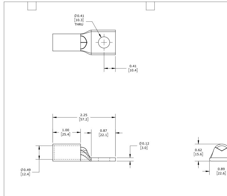
STANDARD BARREL, TIN-PLATED COPPER, 35 KV, 3/8IN MOUNTING BOLT, 1 HOLE, 3/0 AWG, ORANGE MARKINGS.
