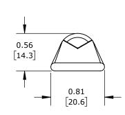
STANDARD BARREL, TIN-PLATED COPPER, 35 KV, 5/16IN MOUNTING BOLT, 1 HOLE, 2/0 AWG, BLACK MARKINGS.
