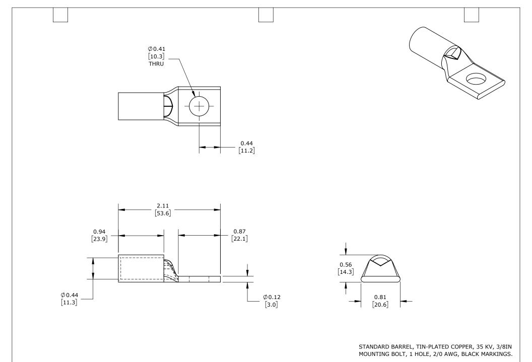
BLU-2\_0S-1 AutomationDirect.com PENN UNION COMPRESSION LUG 1-800-633-0405 PART DIMENSIONS MAY DIFFER SLIGHTLY UNLESS OTHERWISE LATEST VERSION NOT TO INCH UNITS USED FOR inch 3rd SHEET 1 OF 1 SPECIFIED UNITS ARE: ANGLE DUE TO MANUFACTURER'S VARIANCES [mm] 9/9/2024 SCALE PART DESIGN
