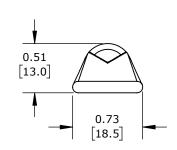
STANDARD BARREL, TIN-PLATED COPPER, 35 KV, 3/8IN MOUNTING BOLT, 1 HOLE, 1/0 AWG, PINK MARKINGS.
