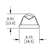
STANDARD BARREL, TIN-PLATED COPPER, 35 KV, 5/16IN MOUNTING BOLT, 1 HOLE, 1/0 AWG, PINK MARKINGS.
