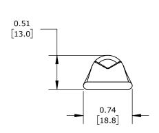
STANDARD BARREL, TIN-PLATED COPPER, 35 KV, 1/4IN MOUNTING BOLT, 2 HOLE, 0.63IN HOLE SPACING, 1/0 AWG, PINK MARKINGS.
