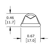
STANDARD BARREL, TIN-PLATED COPPER, 35 KV, 3/8IN MOUNTING BOLT, 1 HOLE, 1 AWG, GREEN MARKINGS.
