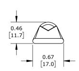
STANDARD BARREL, TIN-PLATED COPPER, 35 KV, 5/16IN MOUNTING BOLT, 1 HOLE, 1 AWG, GREEN MARKINGS.
