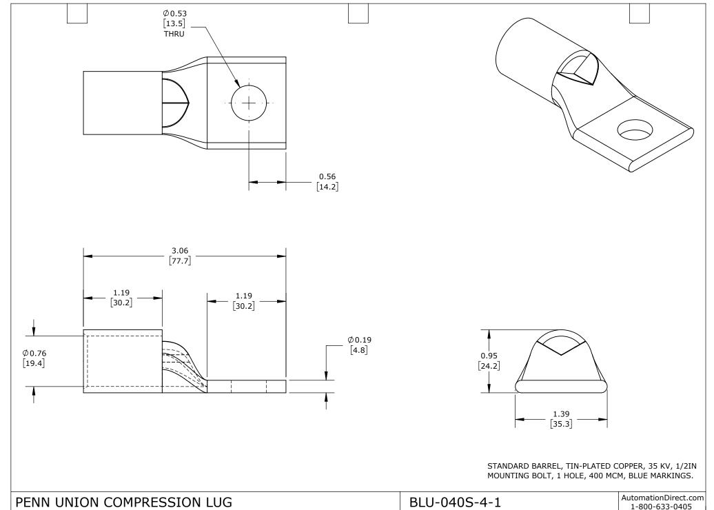
3rd NOT TO PART DIMENSIONS MAY DIFFER SLIGHTLY INCH UNITS USED FOR UNLESS OTHERWISE Inch LATEST VERSION SHEET 1 OF 1
