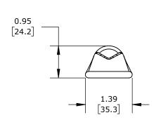
STANDARD BARREL, TIN-PLATED COPPER, 35 KV, 1/2IN MOUNTING BOLT, 2 HOLE, 1.75IN HOLE SPACING, 400 MCM, BLUE MARKINGS.
