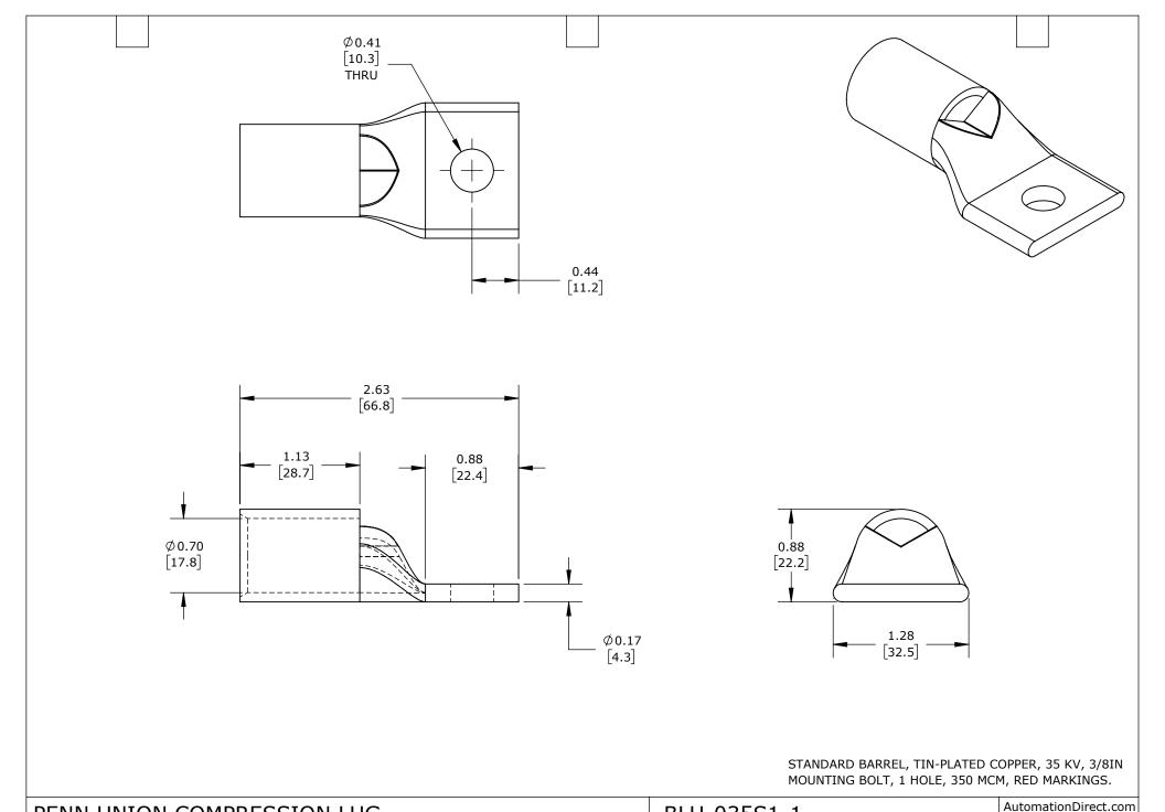
PENN UNION COMPRESSION LUG BLU-035S1-1 1-800-633-0405 PART DIMENSIONS MAY DIFFER SLIGHTLY UNLESS OTHERWISE LATEST VERSION INCH UNITS USED FOR inch 3rd NOT TO SHEET 1 OF 1 SPECIFIED UNITS ARE: ANGLE DUE TO MANUFACTURER'S VARIANCES [mm] 9/9/2024 SCALE PART DESIGN
