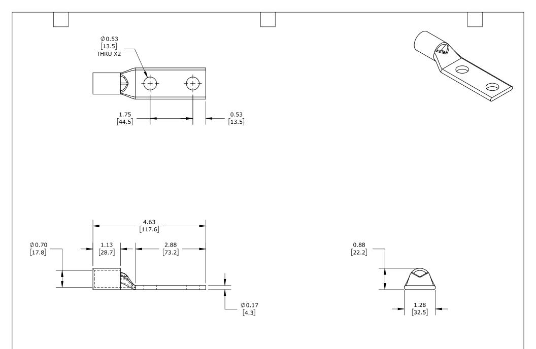
STANDARD BARREL, TIN-PLATED COPPER, 35 KV, 1/2IN MOUNTING BOLT, 2 HOLE, 1.75IN HOLE SPACING, 350 MCM, RED MARKINGS.
