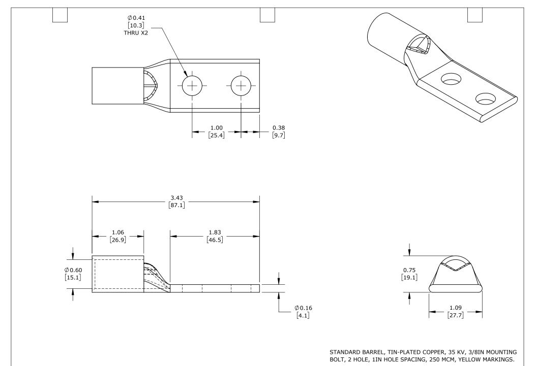
AutomationDirect.com PENN UNION COMPRESSION LUG BLU-025D-2TC38-1 1-800-633-0405 PART DIMENSIONS MAY DIFFER SLIGHTLY UNLESS OTHERWISE LATEST VERSION INCH UNITS USED FOR inch 3rd NOT TO SHEET 1 OF 1 SPECIFIED UNITS ARE: ANGLE DUE TO MANUFACTURER'S VARIANCES [mm] 9/9/2024 SCALE PART DESIGN
