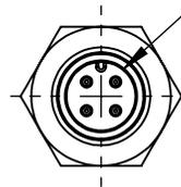
BALLUFF CAPACITIVE PROXIMITY SENSOR, TUBULAR, 12MM DIAMETER X 60MM BODY, STAINLESS STEEL HOUSING, NPN/PNP, N.C., 5MM SENSING DISTANCE, FLUSH, 100 HZ SWITCHING FREQUENCY, IP67, 4-PIN M12 QUICK-DISCONNECT.
