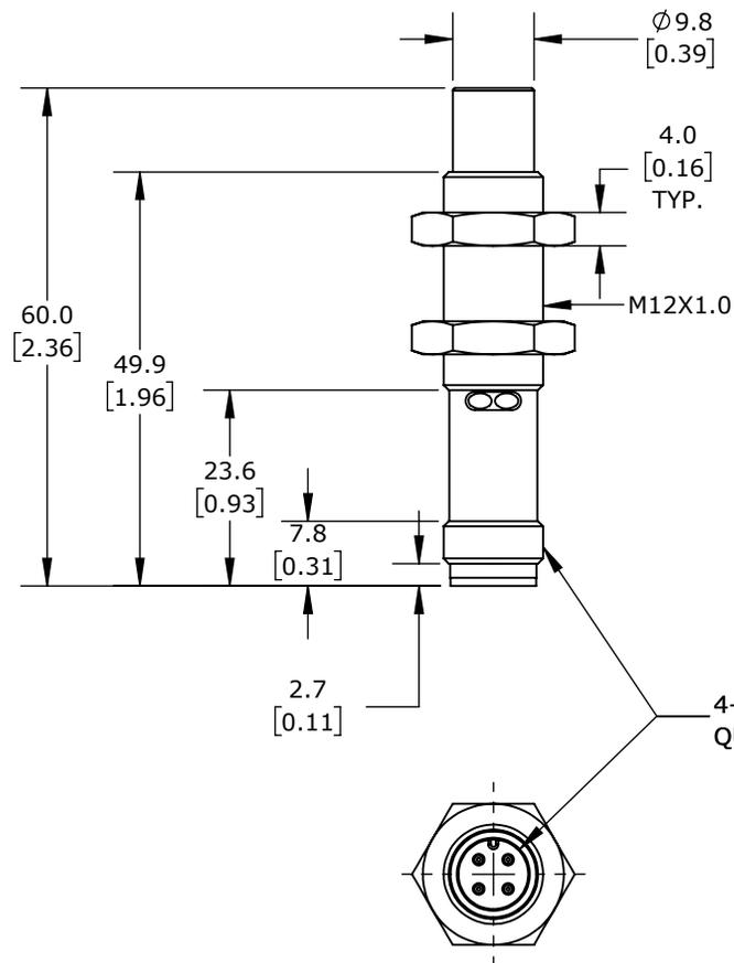
BALLUFF CAPACITIVE PROXIMITY SENSOR, TUBULAR, 12MM DIAMETER X 60MM BODY, STAINLESS STEEL HOUSING, NPN/PNP, N.C., 8MM SENSING DISTANCE, NON-FLUSH, 100 HZ SWITCHING FREQUENCY, IP67, 4-PIN M12 QUICK-DISCONNECT.
