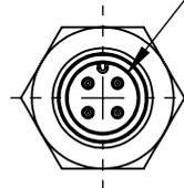
BALLUFF CAPACITIVE PROXIMITY SENSOR, TUBULAR, 12MM DIAMETER X 60MM BODY, STAINLESS STEEL HOUSING, NPN/PNP, N.O., 8MM SENSING DISTANCE, NON-FLUSH, 100 HZ SWITCHING FREQUENCY, IP67, 4-PIN M12 QUICK-DISCONNECT.
