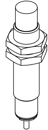
BALLUFF CAPACITIVE PROXIMITY SENSOR, TUBULAR, 12MM DIAMETER X 61MM BODY, POLYBUTYLENE TEREPHTHALATE HOUSING, PNP, N.C., 8MM SENSING DISTANCE, NON-FLUSH, 100 HZ SWITCHING FREQUENCY, IP67, PIGTAIL.
