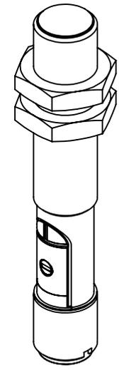
BALLUFF CAPACITIVE PROXIMITY SENSOR, TUBULAR, 12MM DIAMETER X 75MM BODY, STAINLESS STEEL HOUSING, PNP, N.O., 4MM SENSING DISTANCE, FLUSH, 100 HZ SWITCHING FREQUENCY, IP67, 4-PIN M12 QUICK-DISCONNECT.
