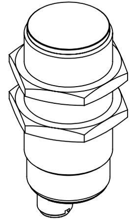
BALLUFF CAPACITIVE PROXIMITY SENSOR, TUBULAR, 30MM DIAMETER X 79MM BODY, POLYBUTYLENE TEREPHTHALATE HOUSING, PNP, N.O., 15MM SENSING DISTANCE, FLUSH, 100 HZ SWITCHING FREQUENCY, IP67, 4-PIN M12 QUICK-DISCONNECT.
