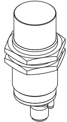
BALLUFF CAPACITIVE PROXIMITY SENSOR, TUBULAR, 30MM DIAMETER X 86.5MM BODY, STAINLESS STEEL HOUSING, PNP, N.O./N.C. SELECTABLE, 30MM SENSING DISTANCE, NON-FLUSH, 100 HZ SWITCHING FREQUENCY, IP66, 4-PIN M12 QUICK-DISCONNECT.
