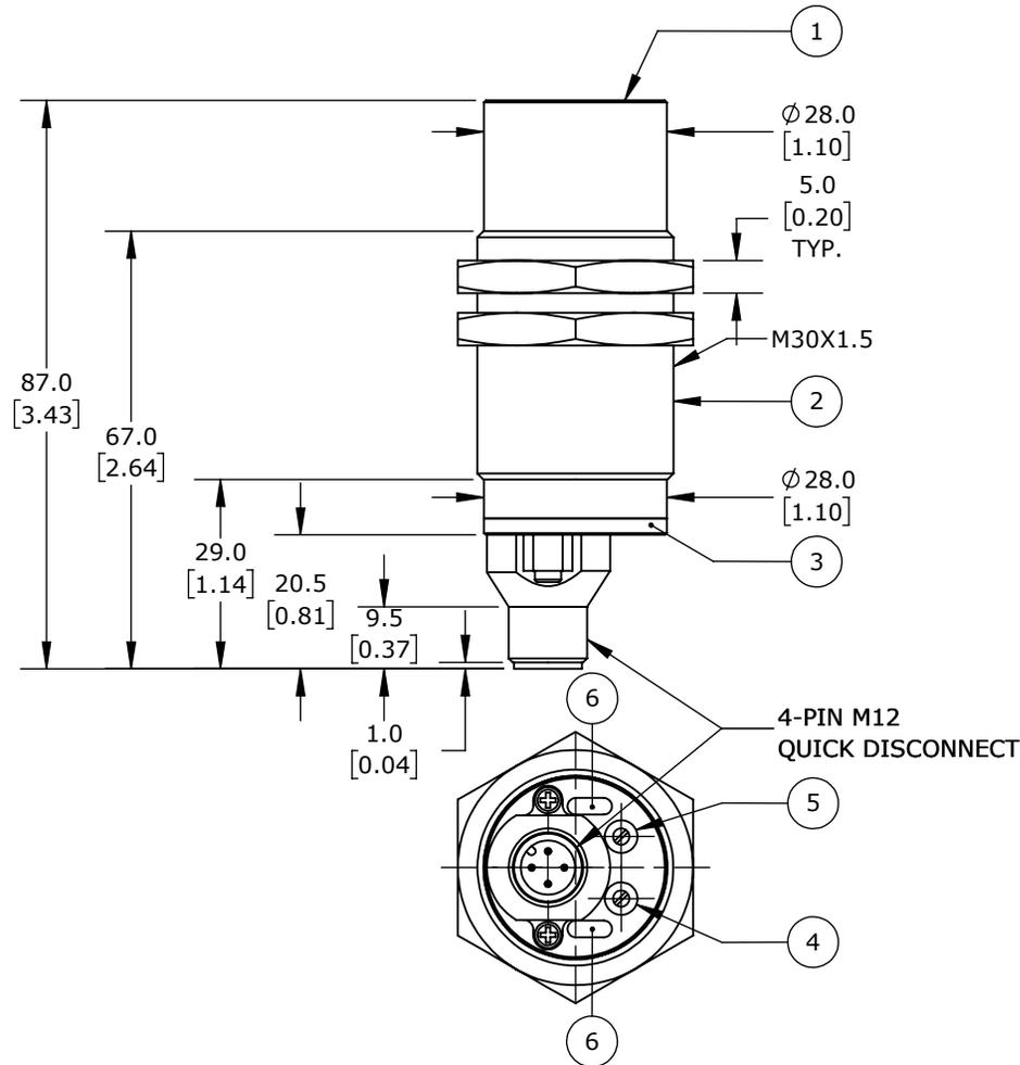
BALLUFF CAPACITIVE PROXIMITY SENSOR, TUBULAR, 30MM DIAMETER X 87MM BODY, POLYBUTYLENE TEREPHTHALATE HOUSING, PNP, N.O./N.C. SELECTABLE, 30MM SENSING DISTANCE, NON-FLUSH, 100 HZ SWITCHING FREQUENCY, IP66, 4-PIN M12 QUICK-DISCONNECT.
