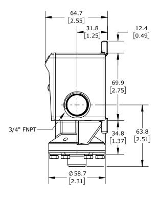
ASHCROFT MECHANICAL PRESSURE SWITCH, 60 TO 400 PSIG SET POINT, 7.0 TO 33.6 PSIG DEADBAND RANGE, VITON SENSING ELEMENT, VITON SEAL(s), SPDT 15A, 1/4IN FEMALE NPT PROCESS CONNECTION, 3/4IN FEMALE NPT CONDUIT OPENING
