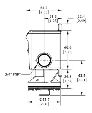
ASHCROFT MECHANICAL PRESSURE SWITCH, 30 TO 200 PSIG SET POINT, 7.0 TO 18.2 PSIG DEADBAND RANGE, VITON SENSING ELEMENT, VITON SEAL(s), SPDT 15A, 1/4IN FEMALE NPT PROCESS CONNECTION, 3/4IN FEMALE NPT CONDUIT OPENING
