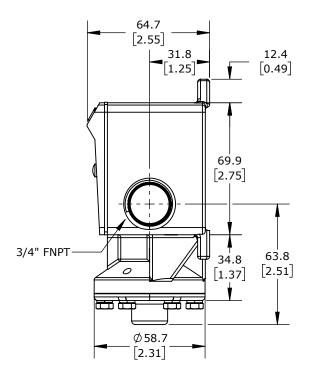
ASHCROFT MECHANICAL PRESSURE SWITCH, 2.25 TO 15 PSIG SET POINT, 0.7 TO 2.1 PSIG DEADBAND RANGE, VITON SENSING ELEMENT, VITON SEAL(s), SPDT 15A, 1/4IN FEMALE NPT PROCESS CONNECTION, 3/4IN FEMALE NPT CONDUIT OPENING
