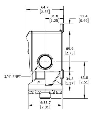
ASHCROFT MECHANICAL PRESSURE SWITCH, 60 TO 400 PSIG SET POINT, 5 TO 24 PSIG DEADBAND RANGE, BUNA-N SENSING ELEMENT, BUNA-N SEAL(s), SPDT 15A, 1/4IN FEMALE NPT PROCESS CONNECTION, 3/4IN FEMALE NPT CONDUIT OPENING
