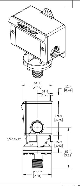
ASHCROFT MECHANICAL PRESSURE SWITCH, 450 TO 3000 PSIG SET POINT, 80 TO 235 PSIG DEADBAND RANGE, BUNA-N SENSING ELEMENT, BUNA-N SEAL(s), SPDT 15A, 1/2IN MALE NPT OR 1/4IN FEMALE NPT PROCESS CONNECTION, 3/4IN FEMALE NPT CONDUIT
