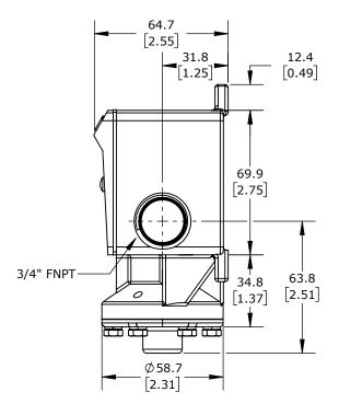
ASHCROFT MECHANICAL PRESSURE SWITCH, 4.5 TO 30 PSIG SET POINT, 0.5 TO 1.5 PSIG DEADBAND RANGE, BUNA-N SENSING ELEMENT, BUNA-N SEAL(s), SPDT 15A, 1/4IN FEMALE NPT PROCESS CONNECTION, 3/4IN FEMALE NPT CONDUIT OPENING
