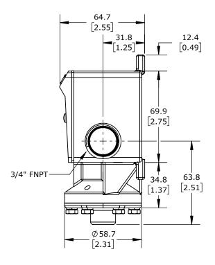
ASHCROFT MECHANICAL PRESSURE SWITCH, 30 TO 200 PSIG SET POINT, 5 TO 13 PSIG DEADBAND RANGE, BUNA-N SENSING ELEMENT, BUNA-N SEAL(s), SPDT 15A, 1/4IN FEMALE NPT PROCESS CONNECTION, 3/4IN FEMALE NPT CONDUIT OPENING
