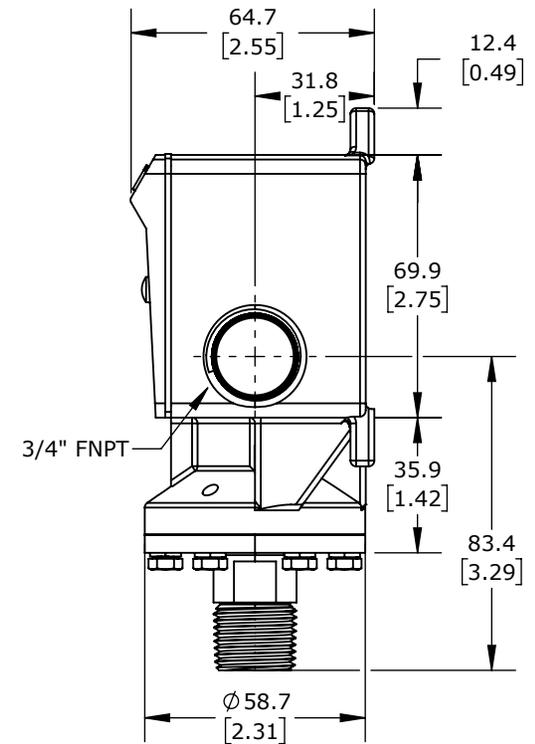
ASHCROFT MECHANICAL PRESSURE SWITCH, 150 TO 1000 PSIG SET POINT, 30 TO 110 PSIG DEADBAND RANGE, BUNA-N SENSING ELEMENT, BUNA-N SEAL(S), SPDT 15A, 1/2IN MALE NPT OR 1/4IN FEMALE NPT PROCESS CONNECTION, 3/4IN FEMALE NPT CONDUIT
