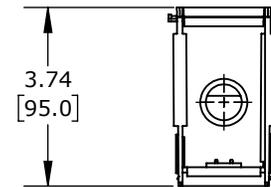
FINGER-SAFE, 310A, 1-POLE, LINE SIDE: 1 OPENINGS ACCEPT 350 MCM TO 6 AWG CU/AL, LOAD SIDE: 1 OPENINGS ACCEPT 350 MCM TO 6 AWG CU/AL, DIN RAIL OR PANEL MOUNT, UL 1953 LISTED.
