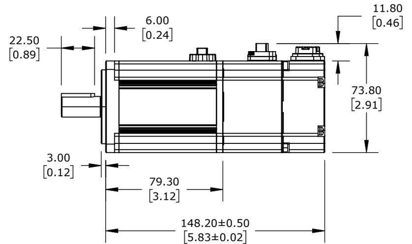
LS ELECTRIC LOW INERTIA DC BRUSHLESS SERVO MOTOR, 300W, 3-PHASE INPUT, 19-BIT (524288 PPR)
