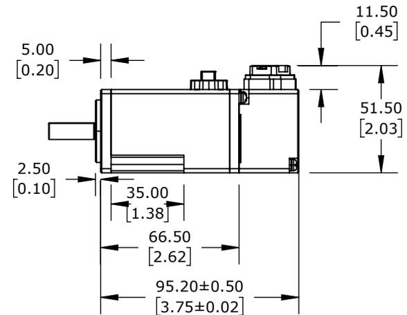
LS ELECTRIC LOW INERTIA DC BRUSHLESS SERVO MOTOR, 100W, 3-PHASE INPUT, 18-BIT (262144 PPR)
