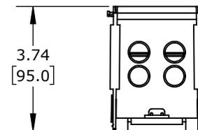
FINGER-SAFE, 760A, 1-POLE, LINE SIDE: 2 OPENINGS ACCEPT 500 MCM TO 4 AWG CU/AL, LOAD SIDE: 4 OPENINGS ACCEPT 4/0 AWG TO 6 AWG CU/AL, DIN RAIL OR PANEL MOUNT, UL 1953 LISTED.
