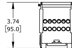
FINGER-SAFE, 760A, 1-POLE, LINE SIDE: 2 OPENINGS ACCEPT 500 MCM TO 4 AWG CU/AL, LOAD SIDE: 12 OPENINGS ACCEPT 4 AWG TO 14 AWG CU/AL, DIN RAIL OR PANEL MOUNT, UL 1953 LISTED.
