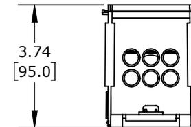
FINGER-SAFE, 380A, 1-POLE, LINE SIDE: 1 OPENINGS ACCEPT 500 MCM TO 4 AWG CU/AL, LOAD SIDE: 6 OPENINGS ACCEPT 2/0 AWG TO 14 AWG CU/AL, DIN RAIL OR PANEL MOUNT, UL 1953 LISTED.
