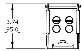
FINGER-SAFE, 380A, 1-POLE, LINE SIDE: 1 OPENINGS ACCEPT 500 MCM TO 4 AWG CU/AL, LOAD SIDE: 4 OPENINGS ACCEPT 4/0 AWG TO 6 AWG CU/AL, DIN RAIL OR PANEL MOUNT, UL 1953 LISTED.
