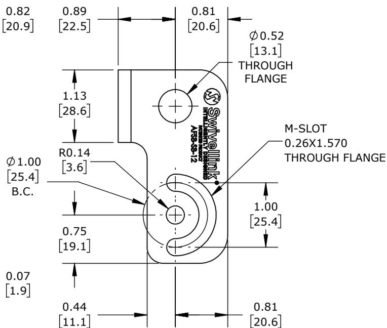
SWIVELINK STANDARD SERIES IMPERIAL SENSOR MOUNT, FOR USE WITH AFSB-SBH, AFSB-SBH-XS AND 12MM THREADED BARREL-TYPE SENSORS.
