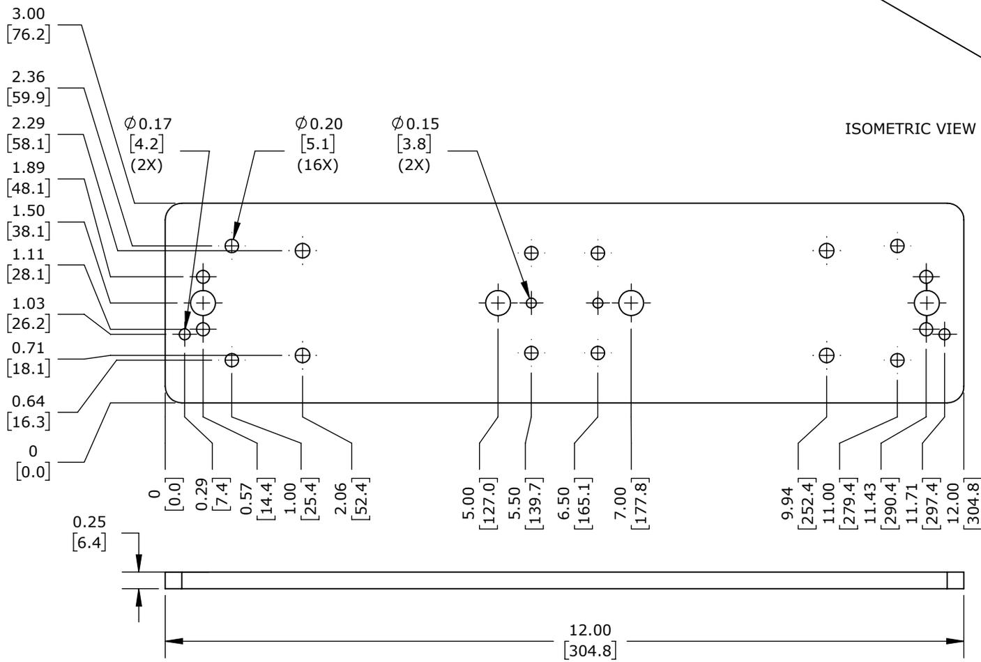
SWIVELINK STANDARD SERIES IMPERIAL MOUNTING PLATE, FOR USE WITH BALL BASES AFSB-1 OR AFSB-1-15 OR AFSB-1XS AND SMART VISION LIGHTS.
