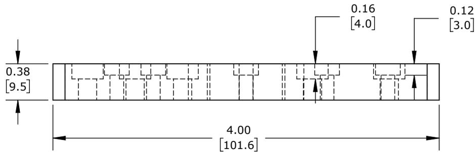
SWIVELINK STANDARD SERIES IMPERIAL MOUNTING PLATE, FOR USE WITH BALL BASES AFSB-1 OR AFSB-1-15 OR AFSB-1XS AND KEYENCE CAMERAS.
