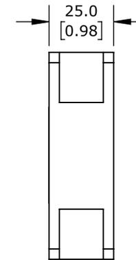
IRONHORSE ACN SERIES MAIN COOLING FAN, REPLACEMENT, 80 X 80 X 25mm, 24 VDC, FOR USE WITH ACN SERIES 15HP - 30HP AC DRIVES
