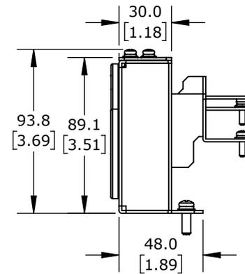
IRONHORSE ACG SERIES CONDUIT BOX, NEMA 1, FOR USE WITH ACG SERIES F FRAME AC DRIVES, MOUNTING HARDWARE INCLUDED
